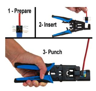
To lock the handles in a parallel position, squeeze the handles slowly together, but not all the way. The handles should stay put.
